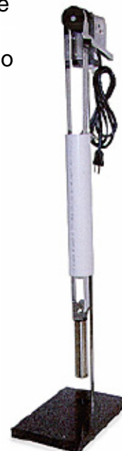
Model MSB Mini-Skimmer™ fitted for a 2" monitoring well. PVC pipe shown on demo model is 2" I.D. fitted with a 1" wide stainless steel belt. Belts can reach as far down as 50 ft. They are equipped with a special small tail pulley and weight bar.
